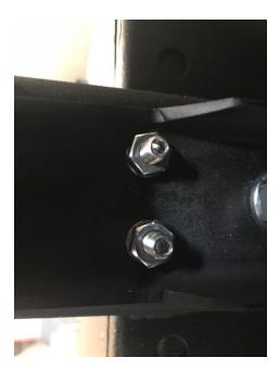
10. Lock down  $\frac{1}{4}$  - 20 set screws with 7/16 wrench while holding set screw in position.
