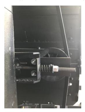
5. Install 3/8 set screw into adjuster plate and attach pulley mount to adjuster plate with supplied 1/2 bolt and leave loose.
