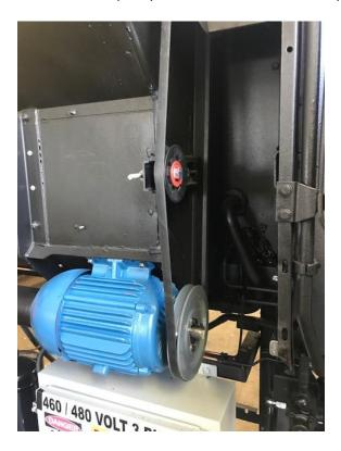
7. Re-install fan shroud and slide fan against shroud to align shroud. Tighten bolts around the fan shroud. Then line mark up on fan with edge of shroud. Tighten fan hub bolts. Re-install access Door.
