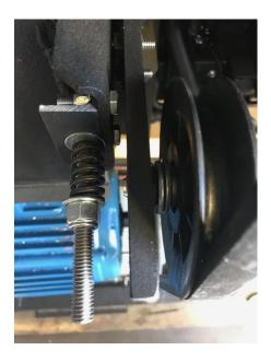
9. If small adjustments are needed, the two ¼ -20 set screws can be used for small lateral adjustments. Bigger adjustments are made by adding or removing washers from between the pulley and pulley mount.
